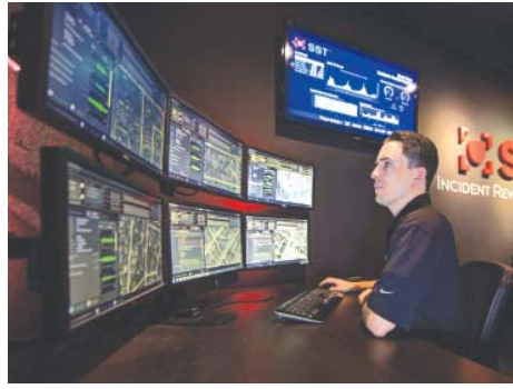
A typical Shotspotter monitoring room, where a technician locates the gunfire on a map and advises the Sheriff's department for a response.
